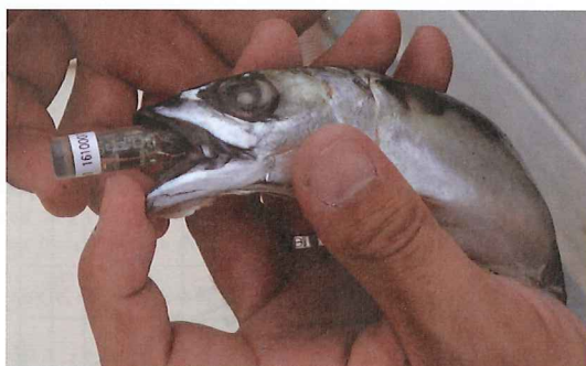
Fig. 3 By letting mackerel swallow the pinger, it was entered the body of a tuna through this bait. As a consequence, wearing of a pinger occurred without injuring the tuna.
